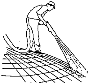
GUNNITE (STANDING ON A BALLOON) HIGH DENSE CONCRETE (POOR INSULATION) DRY MIXTURE CEMENT RICH 15 MM STONE
